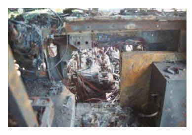
Looking at engine through hole in firewall. Fire started with a wire that grounded out somehow and the voltage melted the plastic and started all the plastic on fire and worked from engine, through firewall, to under dash and spread from there.
