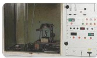
Annex C: Gas analysis in the ISO 5659-2 Smoke Chamber, using FTIR analysis Technique
