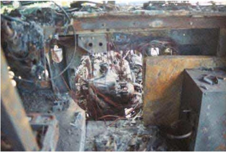
Looking at engine through hole in firewall. Fire started with a wire that grounded out somehow and the voltage melted the plastic and started all the plastic on fire and worked from engine, through firewall, to under dash and spread from there.
