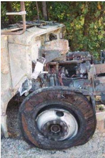
Bus fire started on Passenger side, front tire burned through, Radiator, and most of the engine were melted.
