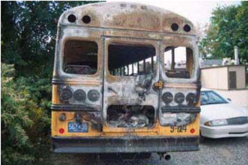
All lights were melted out of the frame. Glass light bulbs melted in the sockets. Glass in the windows melted also.
